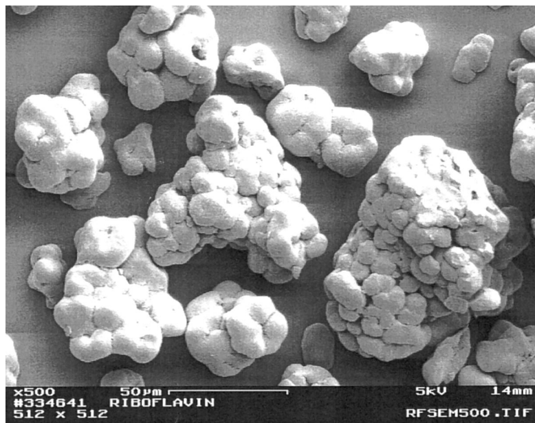
Fig. 2. Scanning electron micrograph of riboflavin sodium phosphate powder. Scale bar = 50 \mu\text{m} .
